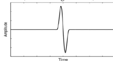
UWB Radar : **High Distance Resolution Capability** (Several cm ~ Several mm)
