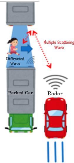
Imaging of Blind Spot by Diffracted Wave and Multiple Scattering Wave
