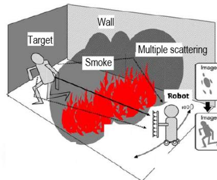
3-dimensional imaging is possible by using the dual-scattering wave synthesis technology as described previously.
