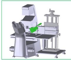
Fig. Microneedle pH sensor indentation units are used under the microscope.
