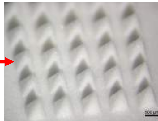
PLA porous MNP composed of bonded microparticles
